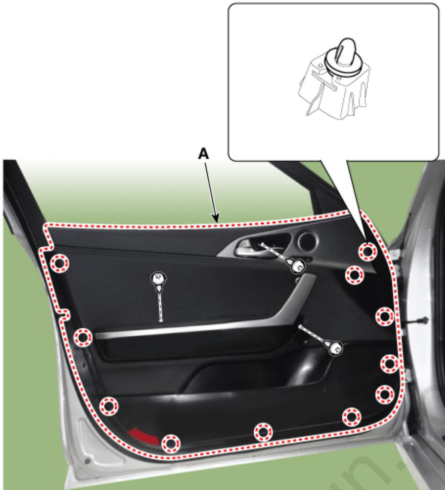
5. Remove the front door inside handle cage (A).
