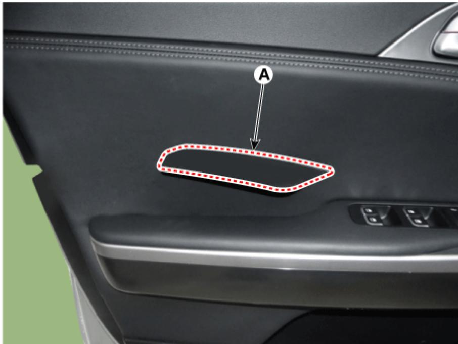
3. Separate the front door inside pull handle mounting cap (A).
