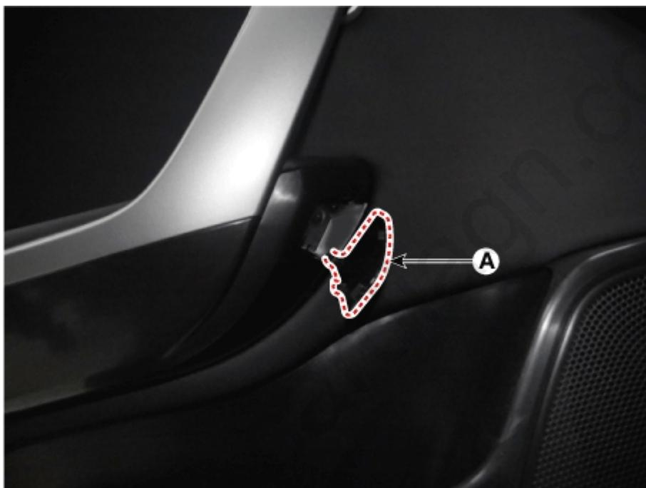
4. Remove the front door trim (A) after loosening the mounting screws.
