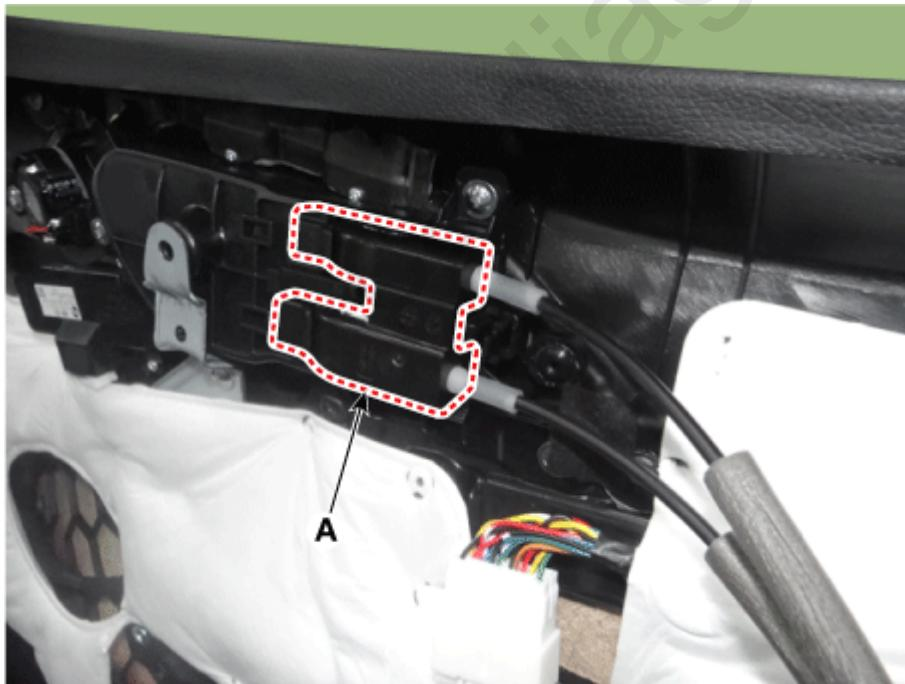
6. Disconnect the front door intergration connector (A).
